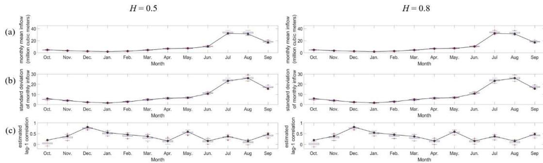
**Figure S4 Monthly statistics of the synthetically generated streamflow series: two cases of  $H = 0.5$  and  $H = 0.8$  with no changes in the annual mean value: (a) monthly mean, (b) standard deviation, and (c) lag-1 correlation.**
