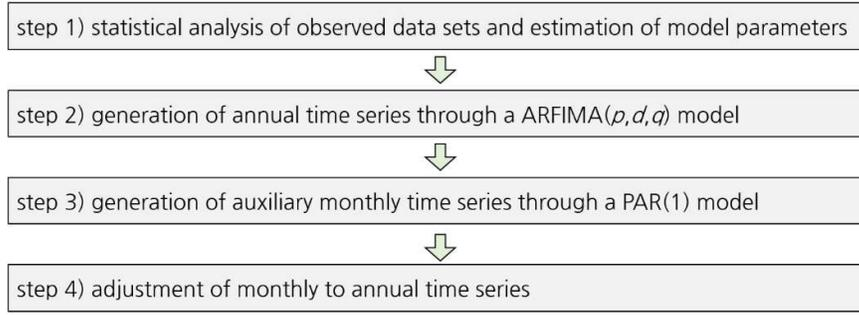
**Figure S1 A flow diagram of stochastic streamflow generation approach.**
